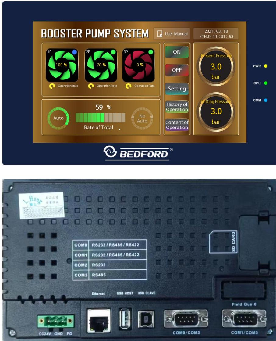
Figure2.1 7 inch touch screen terminal and its introduction
